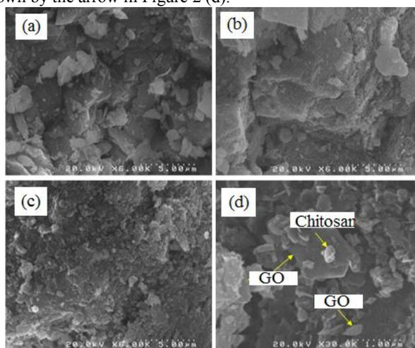
**Figure 2.** FESEM images of the (a) raw, (b) calcined and (c) composite dolomite samples
