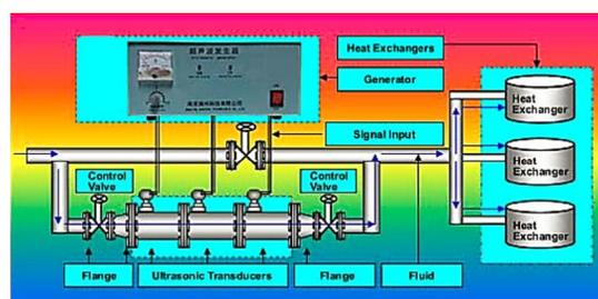
**Figure 1.** The schematic of the anti-precipitation transducer [4]
