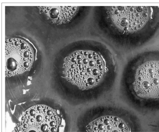
Figure 2. Droplet condensation on the coated part of the substrate and filmwise condensation on the uncoated parts of the same substrate [4].
